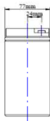
T12 Terminal Unit: mm [inches]
